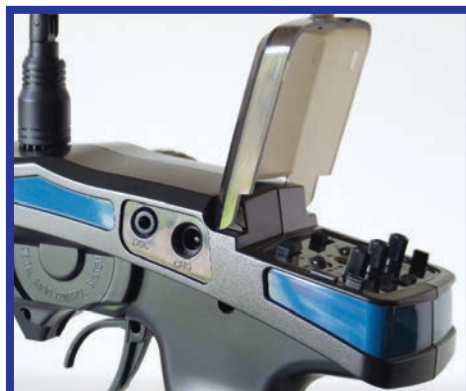
When pulled back to the handset the model should move forwards, if not flick the Throttle switch to the 'Rev' position.
